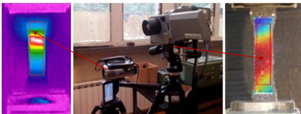
Figure 1. The arrangement of the measuring equipment as well as the deformation zone analyzed by the thermography and DIC methods
