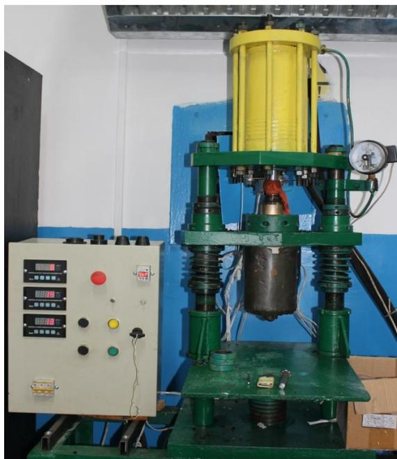
**Figure 4** – PL-32 injection molding machine
