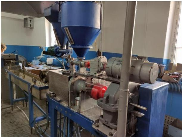
**Figure 3** – Experimental extruder
