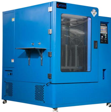
Fig. 2. Typical formaldehyde chamber based on EN 717-1 standard (Guangdong grande automatic test equipment limited, China).
