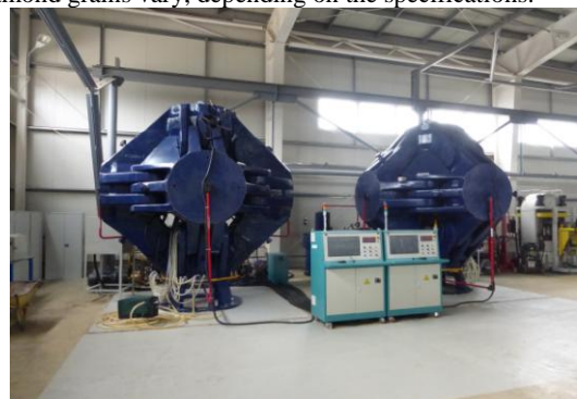
Figure 2. Installations for the manufacture of PDC cutters based on the GY850 multi-punch press.
