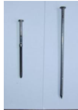
Fig. 3. Comparison of the ordinary and the new nails: a – comparison of the cross-section dimensions; b - view of the used nails with the new shape and \phi 7
