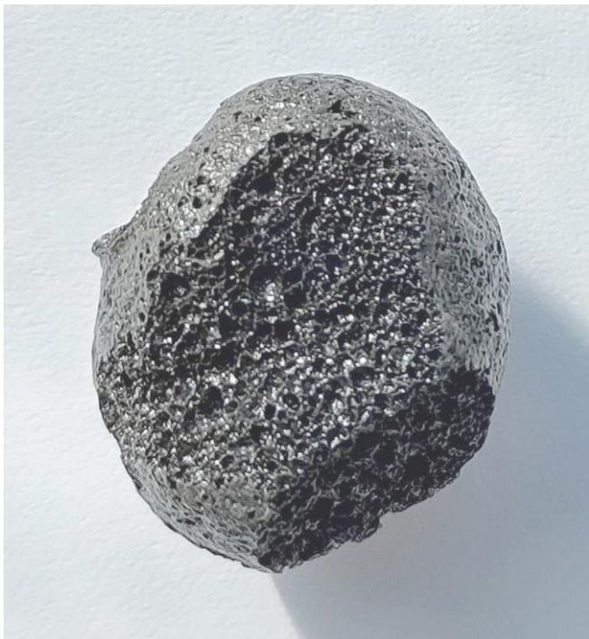
Fig. 3. Foam silicate specimen (horizontal and side section).
