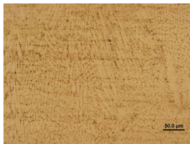
Fig. 10 Microstructure in the area of mixing the cladding metal Dievar and NiCu7
