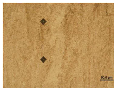
Fig. 7 Microstructure of fist clad layer with Diavar
