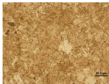
Fig. 5 Microstructure of base material (BM) Dievar
