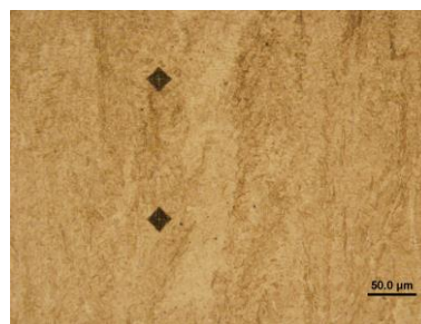
Fig. 7 Microstructure of fist clad layer with Dievar
