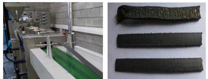
Fig. 5 Experimental investigations of the possibilities of effective production, by plasticizing with extrusion, of new polymer - mineral compositions.
