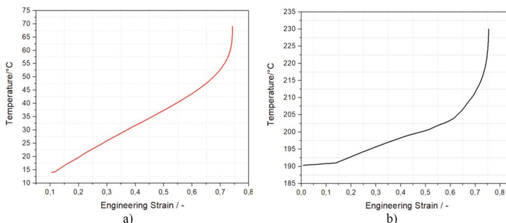
**Figure 4.** The engineering strain-temperature curves for the samples in: a) as cast condition, b) solution hardened condition
