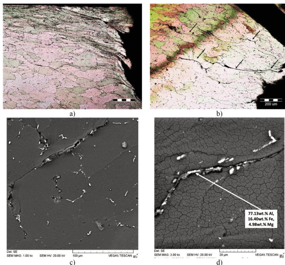
**Figure 7.** The microstructure of the solution hardened sample after compression: a) surface of the sample (Figure 5 b, detail 1), b) progression of the low energy intergranular fracture (Figure 5 b, detail 2), c) grain boundary involvement in fracture progression, d) the Fe-based intermetallic particles located in the fracture
