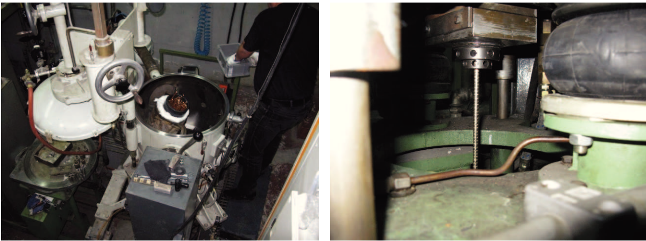
Figure 1 Continuous casting system. (Left) Induction furnace filled with pure Cu and Al rods prepared for melting. (Right) The exit of the as cast rod from the crystallizer.
