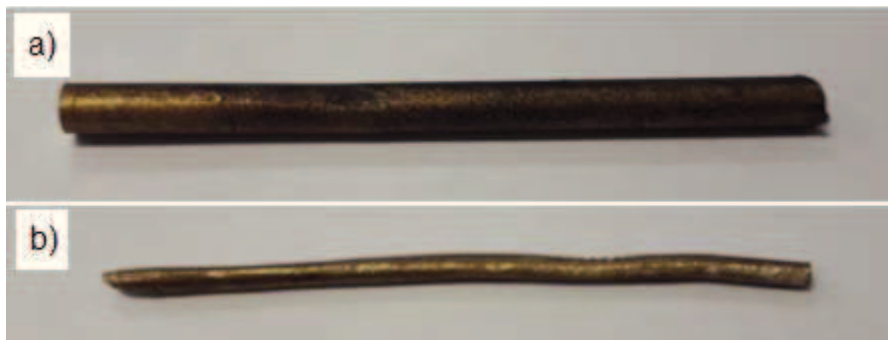
Figure 4. Photograph of CuAlMn shape memory alloy wire \varnothing 4.47 mm (a) and \varnothing 3.22 mm (b)
