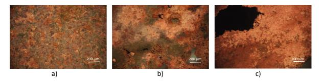
Figure 4. Light microscopy images of the electrode surfaces after potentiodynamic polarization measurements for a) sample A, b) sample B and c) sample C
