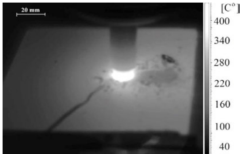
Figure 4. Thermal image of the FSP in run 1
