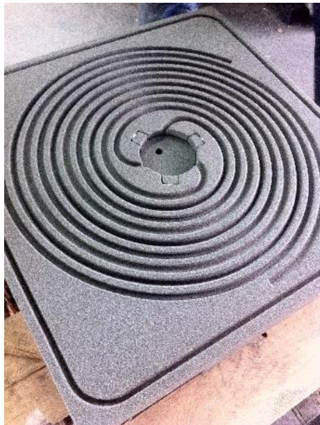
Figure 3. Lower part of the mold made with 3D printing
