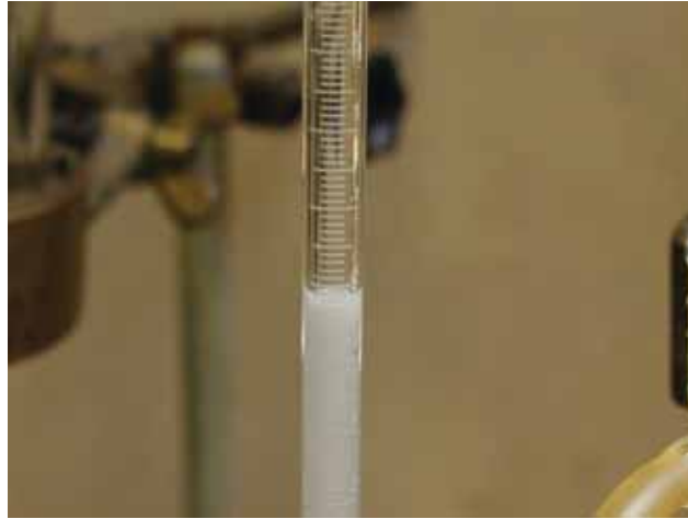
Figure 4. Collecting hydrogen in a measuring tube
