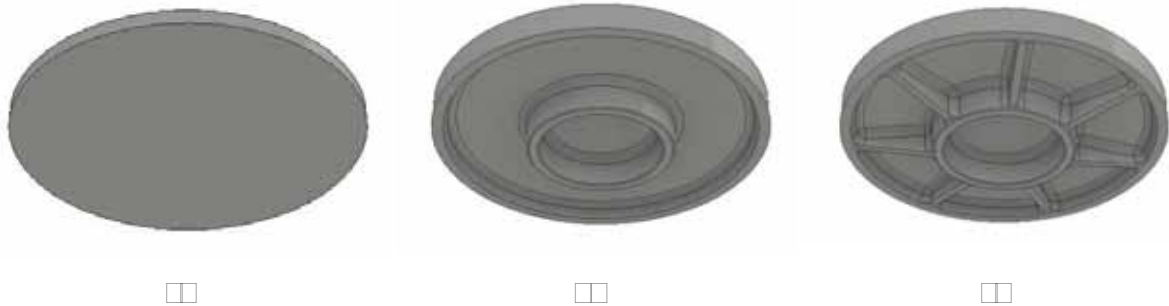
Figure 4. Circular manhole cover: a) Variant I, b) Variant II, c) Variant III
