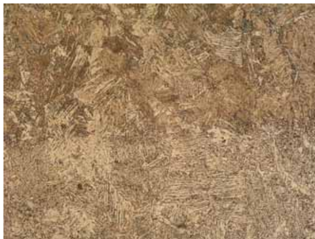
Figure 7. Fusion line – sample IB21, magnification 200 x
