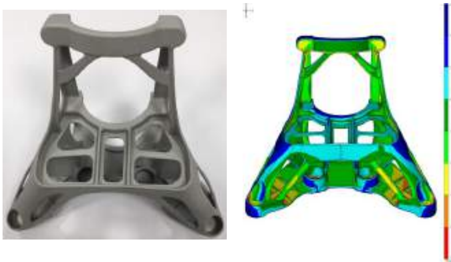
Figure 8. Final casting shape after sand blasting
