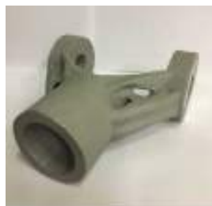
Figure 16. Prototype casting of the hinge after removal of the gating system
