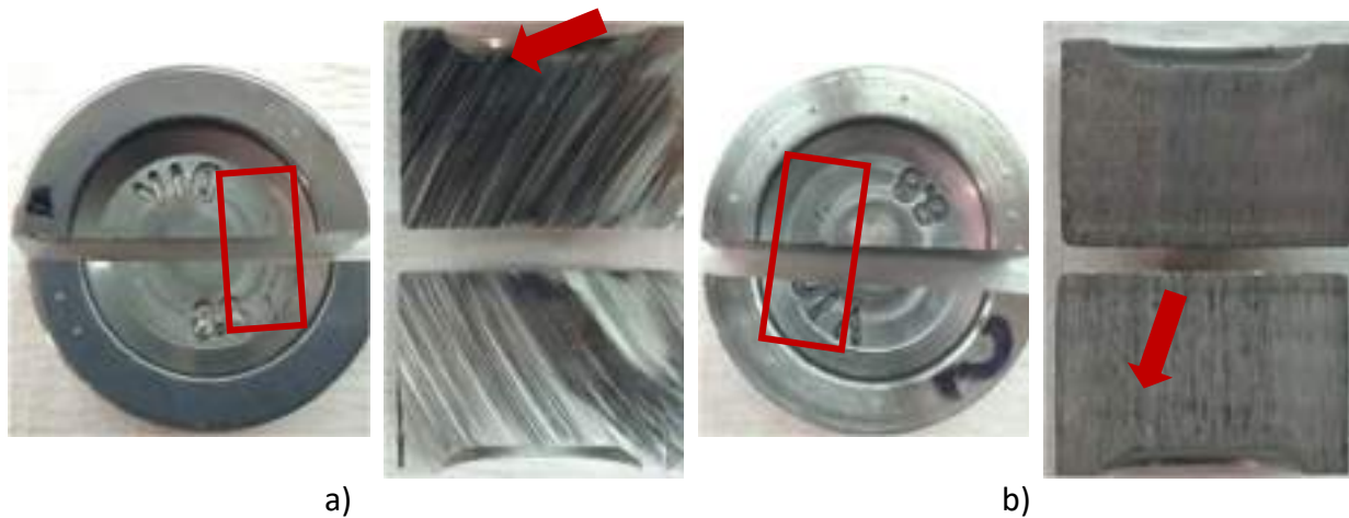
Figure 1. Sampling for metallographic analysis: a) sample 1, b) sample 2
