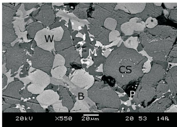
Fig. 1. Scanning electron micrograph (SEM) – wustite (W), calcium silicate (CS), brownmillerite (B), mayenite (M), pores (P) and inclusions of iron (white)
