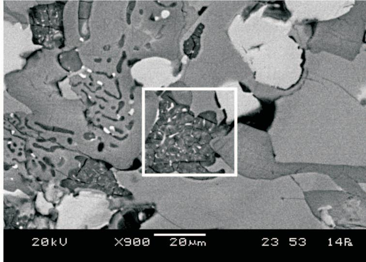
Fig. 3. Scanning electron micrograph (SEM) – the dark grain in the middle of the image is the Mn- mineral
