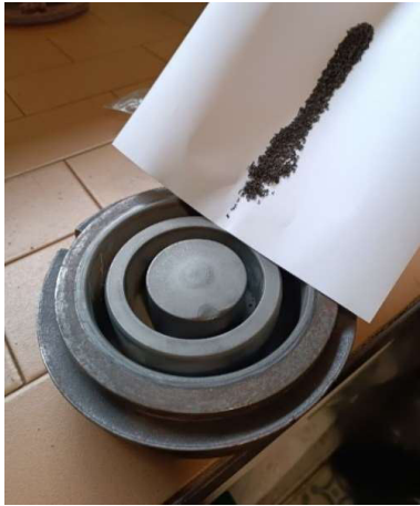
Figure 6. Milling of hydrated TiAl6Nb7 titanium alloy
