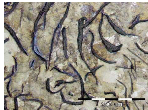
d) etched by nital 2%, magnification 200x
