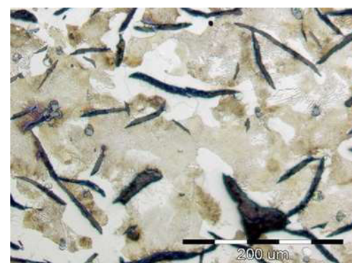
d) etched by nital 2%, magnification 200x
