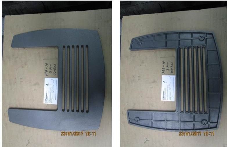
Figure 1. Complex geometry of investigated casting (top nad bottom side)
