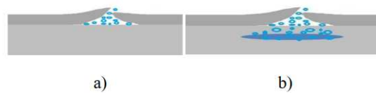
Figure 6. a) hydrogen penetration to the surface, b) separation of the oxide layer [1]
