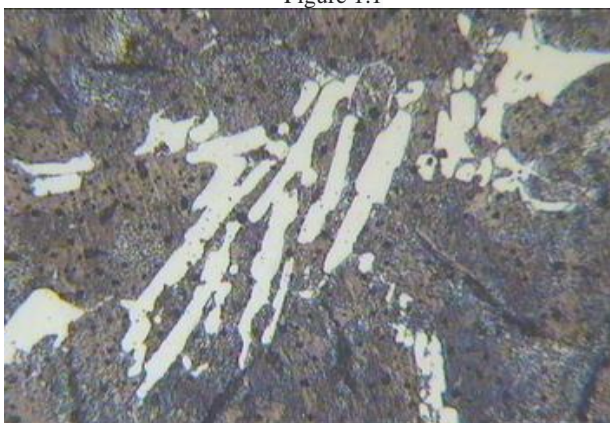
x200- Metal base + carbides + graphite plate Figure 1.2
