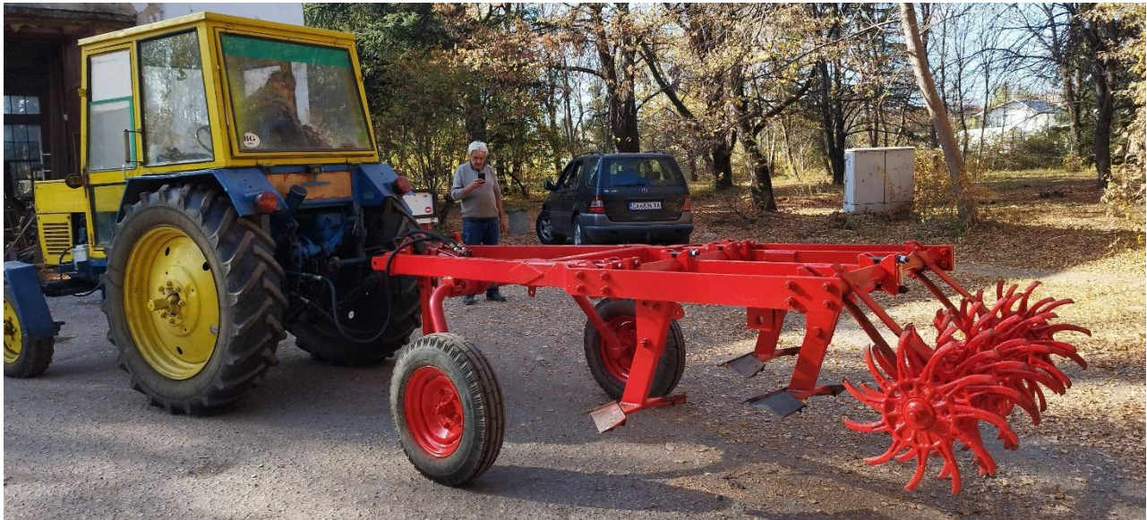
Fig. 3. Trial sample of a combined machine for inter-row processing of perennials in transport position
