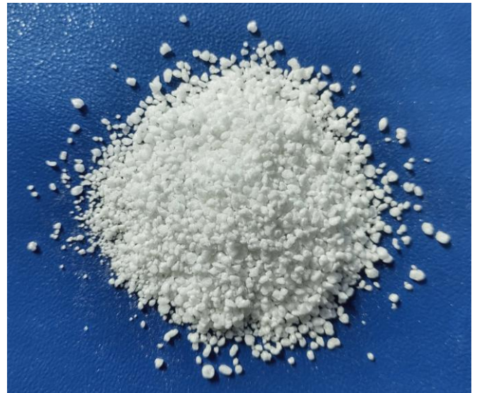
Fig. 1. Perlite for construction (fraction up to 3 mm).
