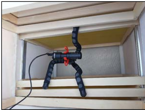
Fig. 2. Installation of the microphone inside the beehive
