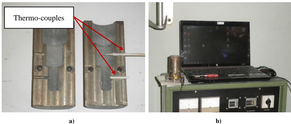
Figure 3.10. Experimental setup for Simplified Thermal Analysis: a) placement of thermo-couple in mold cavity, b) data acquisition instrument
