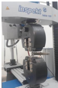
Fig. 3 Static tensile test conducted with extensometer
