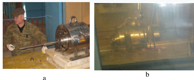
Fig. 5. Preparatory work with recharge container KTP-5M (a) and recharging of the Co-60 source from the emergency holder into a new holder in protective box (b).
