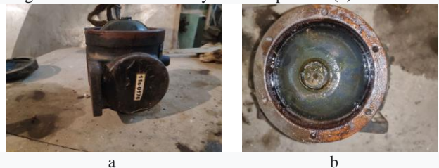
Fig. 7. Depleted uranium container (a) containing a source of Co-60 and a plug of depleted uranium that was completely wedged into the body of the container during expansion (b).
