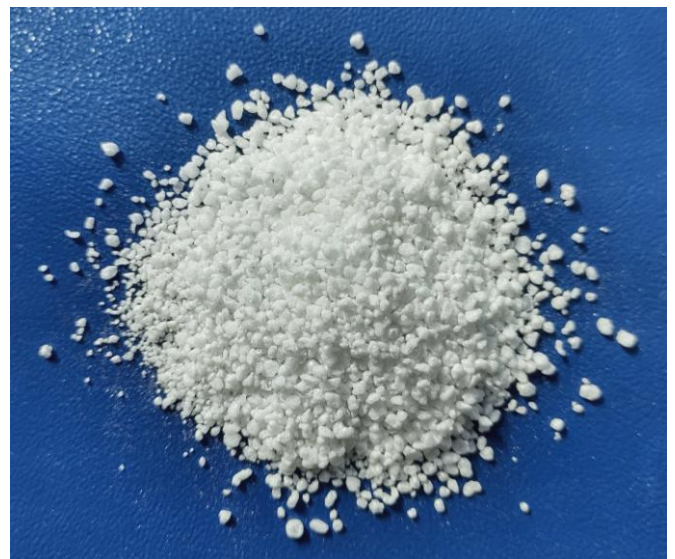
Fig. 1. Perlite for construction (fraction up to 3 mm).
