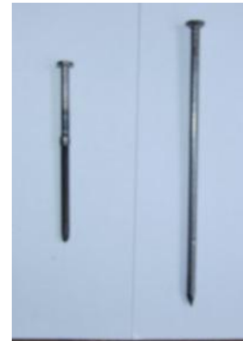
Fig. 3. Comparison of the ordinary and the new nails: a – comparison of the cross-section dimensions; b - view of the used nails with the new shape and φ7
