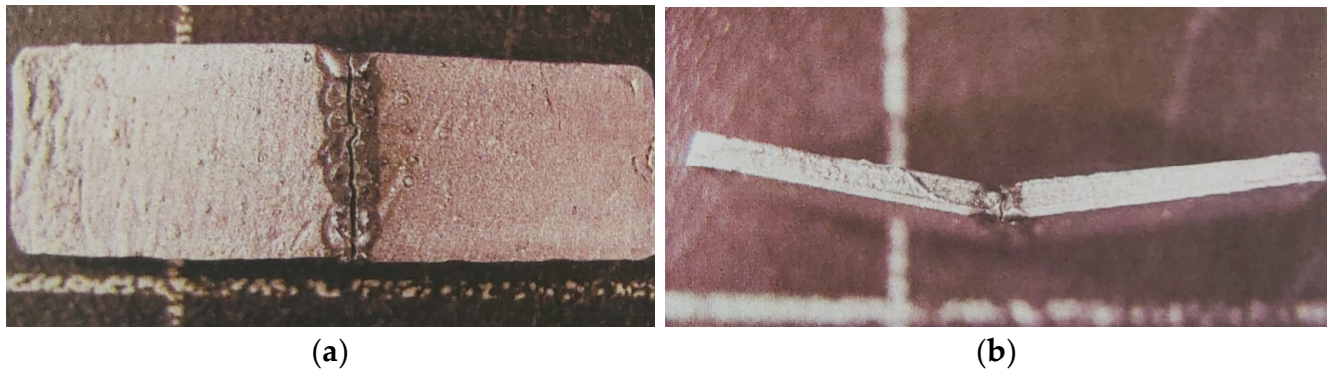
Figure 4. TIG weld of VI-COMP after flexural strength testing. (a) Weld face; (b) Side view of TIG weld.
