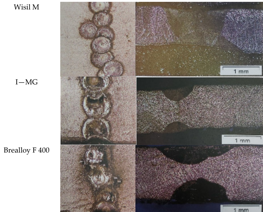
Figure 2. The appearance of the weld face and micrographs of all TIG-welded alloys.
