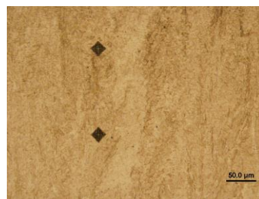
Fig. 7 Microstructure of fist cladded layer with Dievar
