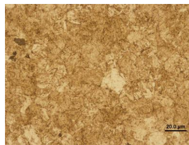
Fig. 5 Microstructure of base material (BM) Dievar
