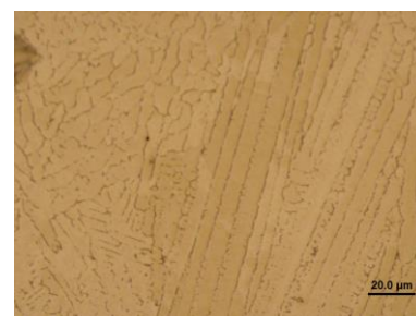
Fig. 8 Microstructure of cover layer cladded with UTP A 702
