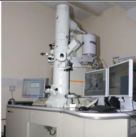
Fig. 1. Multipurpose transmission electron microscope JEOL JEM 2100.
