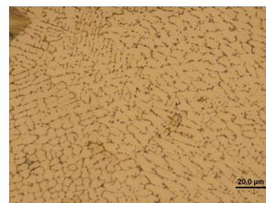
Fig. 9 Microstructure of cover layer cladded with wire NiCu7
