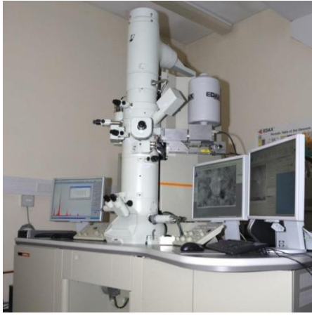
Fig. 1. Multipurpose transmission electron microscope JEOL JEM 2100.
