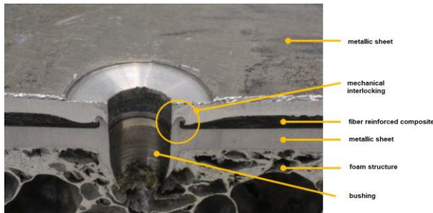
Fig. 16 Metal-composite joints made by Flowdrill method [13]
