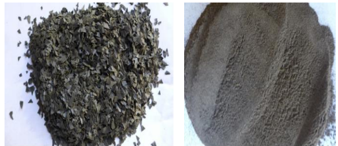
Fig. 4 Appearance of particulate refresher plates and mineral sludge for the production of polymer - mineral composites.
