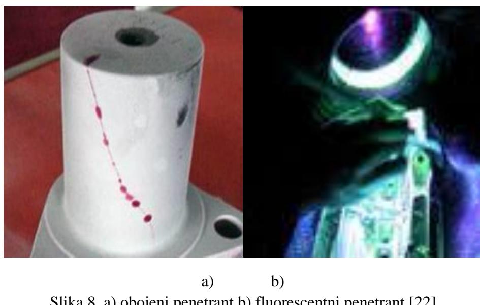
Slika 8. a) obojeni penetrant b) fluorescentni penetrant [22]
