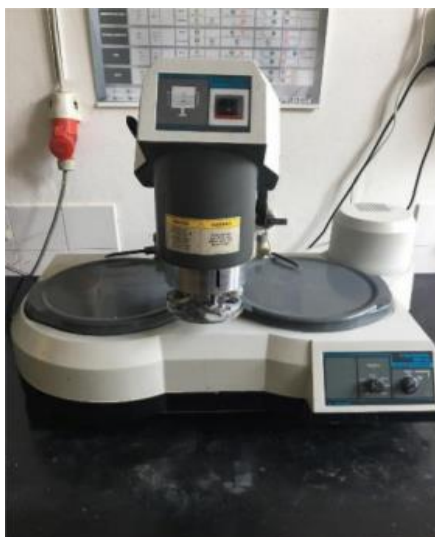
Slika 34. PHOENIX BETA GRINDING/POLISHER s glavom Vector LC
