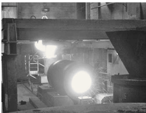
Figure 2 Centrifugal casting of the working shell
