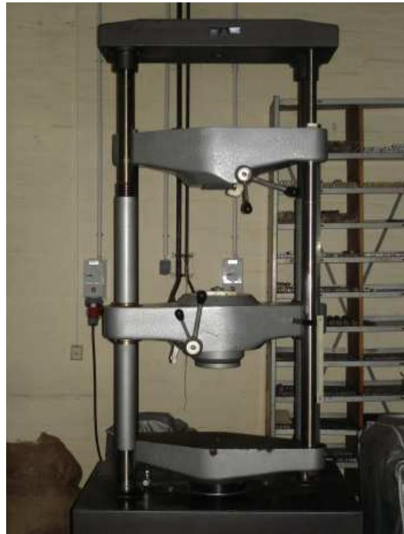
Slika 31. Kidalica WEB WPM/ EUmod/400 kN.
