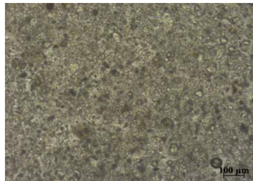
Fig. 7. Microphotography of suspension of alcohol based coatings.
