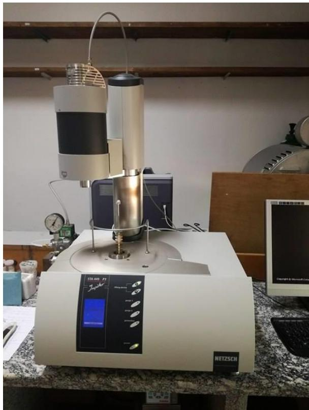
**Slika 14.** Simultani toplinski analizator STA DSC/TG (NETZSCH STA Jupiter 449 F1)
